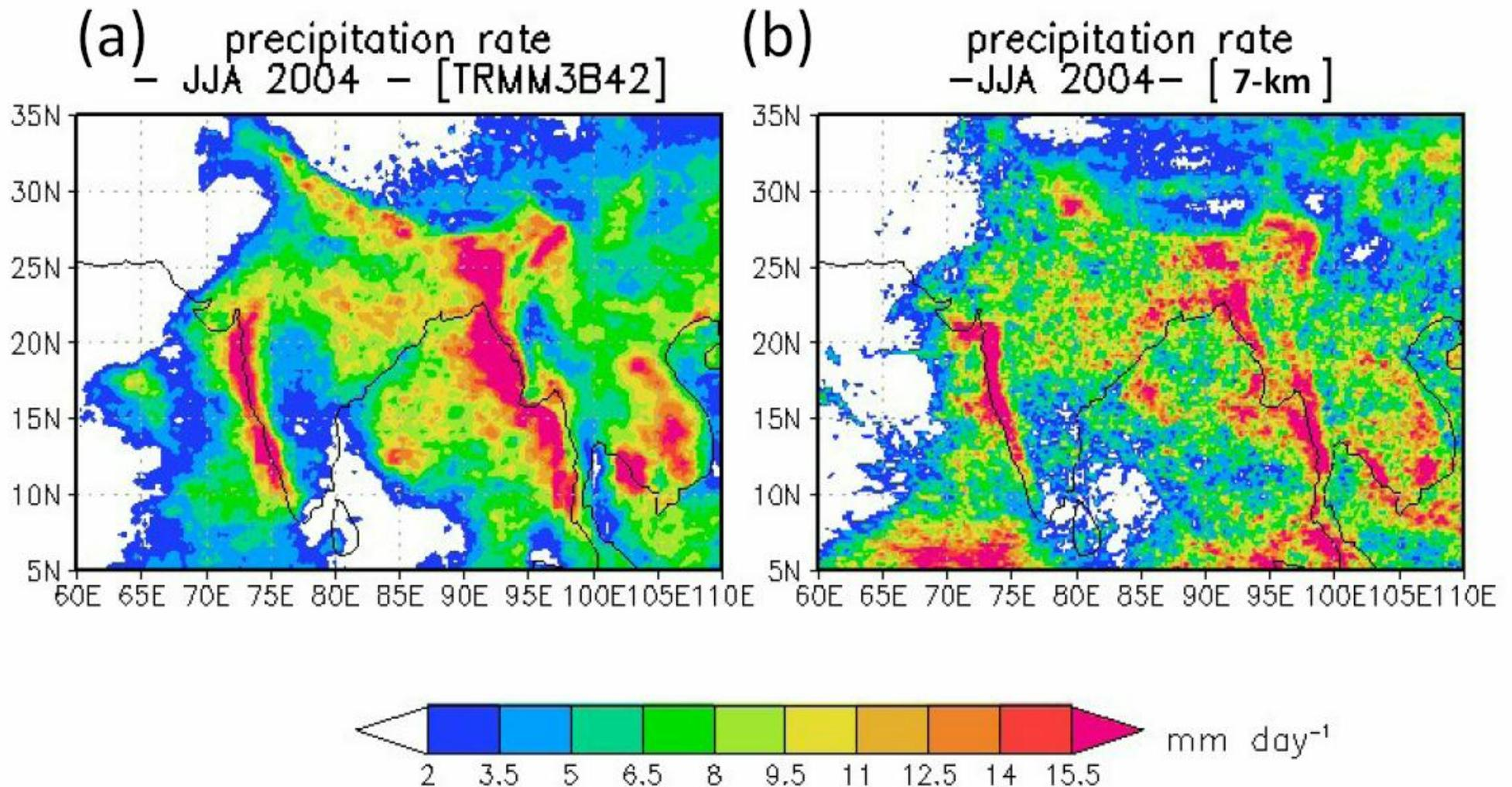
***Oouchi et al. 2009***: (a) Observed and (b) simulated precipitation rate over the Indo-China monsoon region as June-July-August average (in units of mm day<sup>-1</sup>). The observed precipitation is from TRMM\_3B42, and the simulation is for 7km-mesh run.
